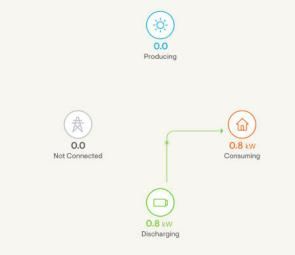
When the grid is down and sunlight is not available, the battery powers the home.
