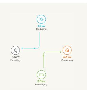
During peak hours, if the export tariff is equal to or higher than the import tariff, the battery powers the home, and the solar production is exported to the grid.
