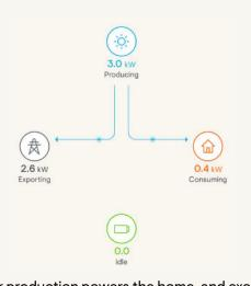
Solar production powers the home, and excess generation is exported to the grid because the battery is fully charged.
