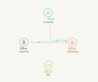
When the battery is fully charged, solar production and grid power the home.
