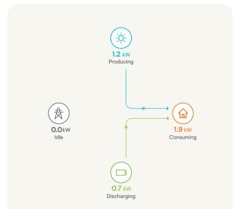
During peak hours, if the export tariff is less than the import tariff, power export is not profitable. Solar production and the battery power the home, minimising power import from the grid.
