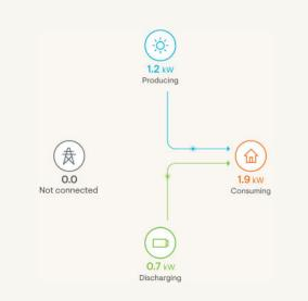
When the grid is down, solar production and battery power the home.
