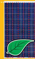
When one half of a standard module is shaded, none of the module produces electricity
