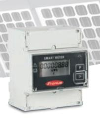
The Fronius Smart Meter is a bidirectional meter, which optimises self-consumption, records the load curve and controls the various energy flows. Thanks to highly accurate measurements and rapid communication via the Modbus RTU interface, dynamic feed-in control when feed-in limits are imposed is faster and more accurate than with the S0 meter.
