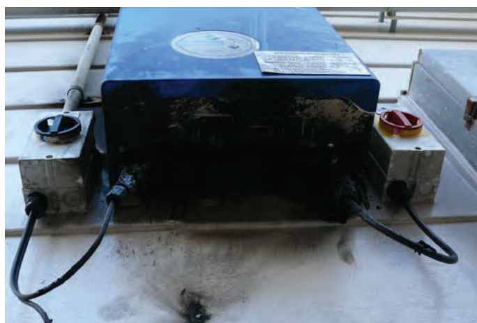
Poor quality inverter - 2 years old
