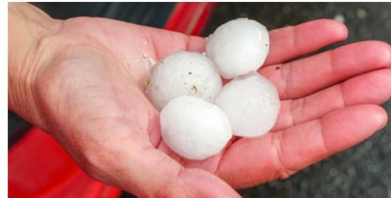
LG panels are tested with larger hailstones (35mm) than standard panels (25mm). The stones in this image are approx 35 mm.
